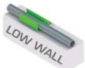
Sealing reinforcement on low wall - ref. 10290
